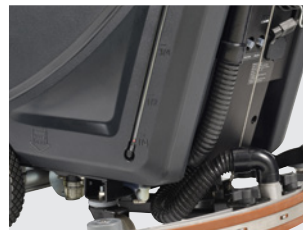
Water level indicator with volume visible on the tank
